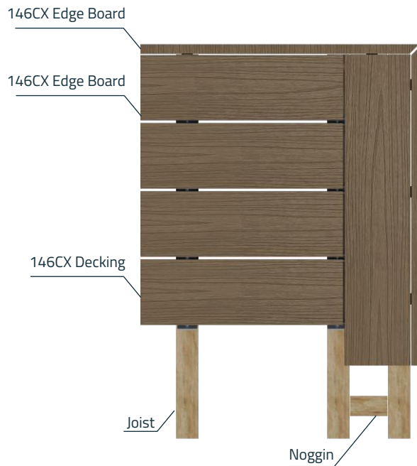
Installed Deck – Top View
