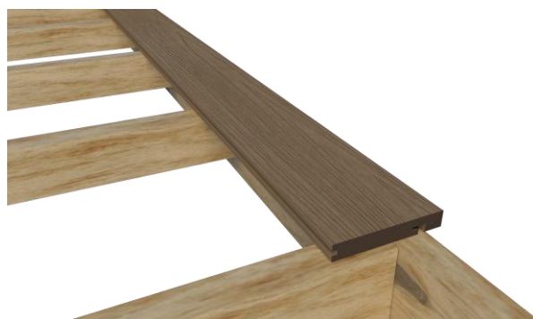
Push the board firmly forward until the groove locks securely into the Start/Stop Clips.
