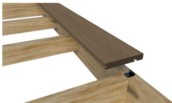
Position the Edge board so the bottom groove lines up with the Start/Stop Clips.
