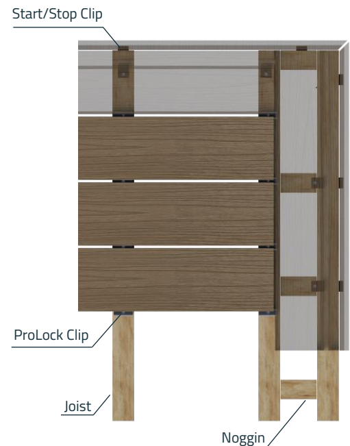
Transparent Deck – Fixing Detail
