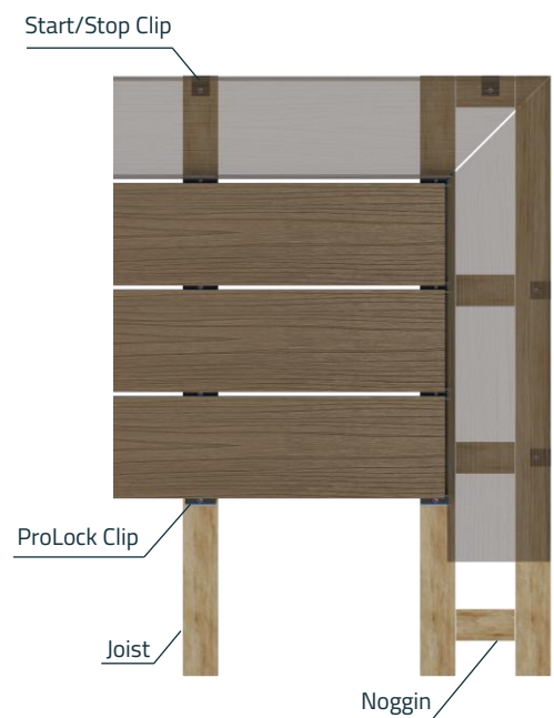
Transparent Deck – Fixing Detail
