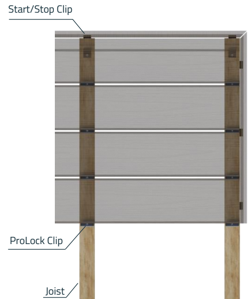
Transparent Deck – Fixing Detail
