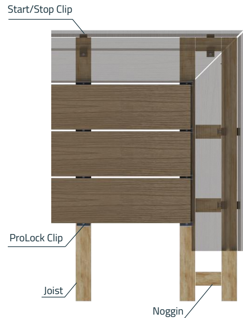
Transparent Deck – Fixing Detail
