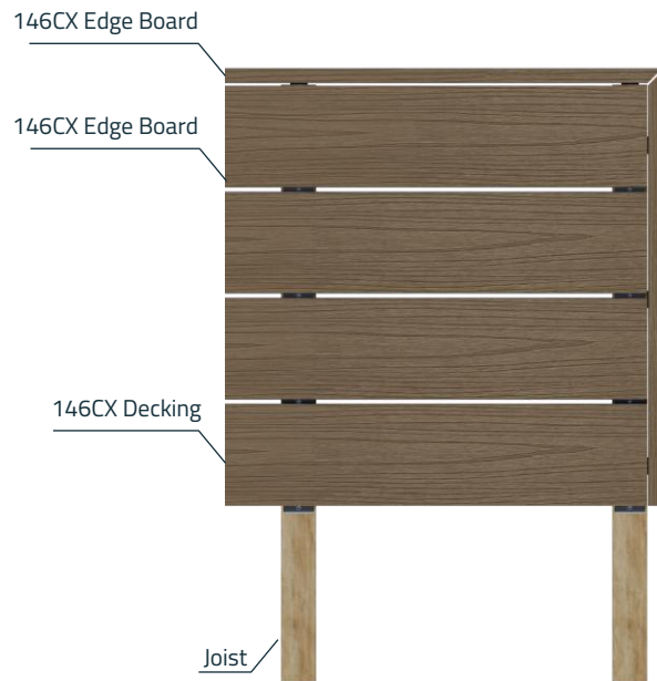
Installed Deck – Top View
