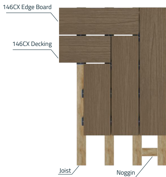
Installed Deck – Top View
