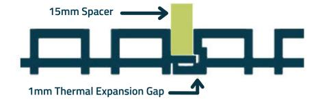
A piece of wood sized to 15mm width can be used as an alternative to a spacer.
