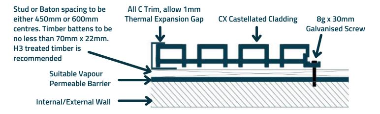
Please note: if the bottom of the Cladding is exposed you will be required to install the PermaTimber® Aluminium Bottom Trim, refer to Page 8 for more information.
