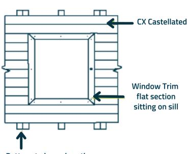
Battens to be no less than 70mm x 22mm H3 Treated Timber with 450 or 600mm centres.
