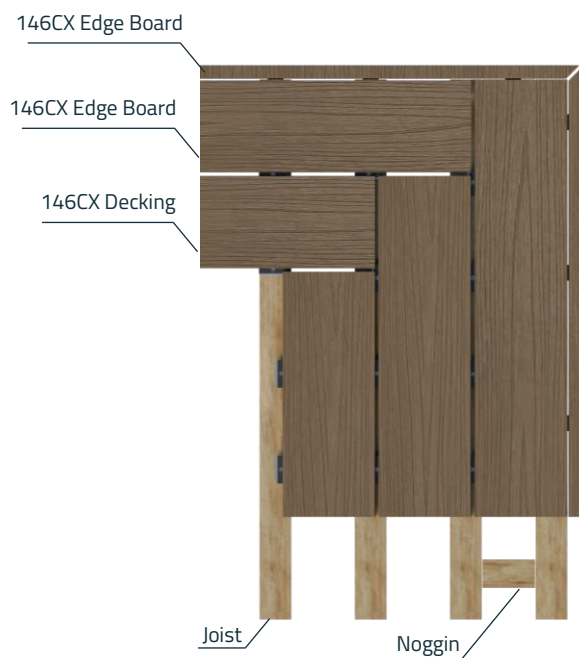
Installed Deck – Top View
