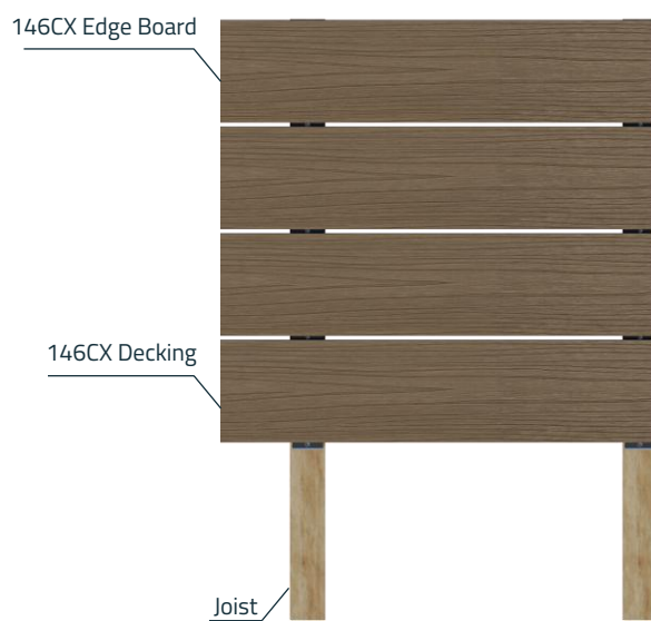
Installed Deck – Top View
