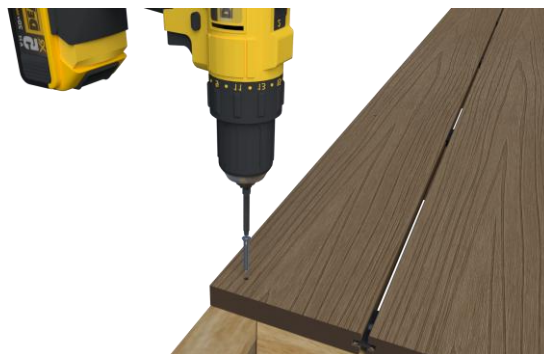
Rip the final board to fit if required, then face fix with oversized, countersunk clearance holes at every joist or maximum 450 mm centres.
