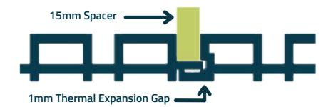
A piece of wood sized to 15mm width can be used as an alternative to a spacer.
