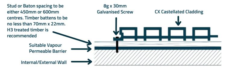
Please Note: CX Castellated Boards must be drilled and fixed with the use of a 15mm spacer to create a 1mm thermal expansion gap between panels.
