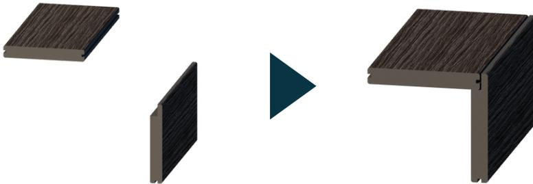
With the edge Board, rip the rebate closest to the bottom of the decking board off. Then attach the decking board lengthways by slotting it into the crevasse. Routing may be needed for the decking board to be flush with the crevasse.
